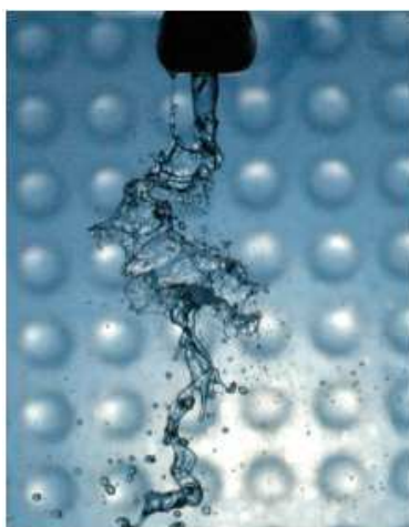
FIG. 15: Example of nozzle wetting and the effect on breakup process.
